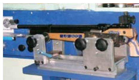
This a custom made vise used at Vogel USA for their pellet testing. It uses round rubber pads to grip the gun at the critical points. It is attached very solidly to the adjacent wall made of 6x6's.
