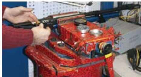
This is the air rifle vise used at the Anschütz factory in Ulm. It is a rather large standard bench vise that is solidly attached to the floor. It has specially shaped jaws that grip the air cylinder and barrel shroud with the stock removed. Note the many strips of tape from thousands of tins of pellets!
