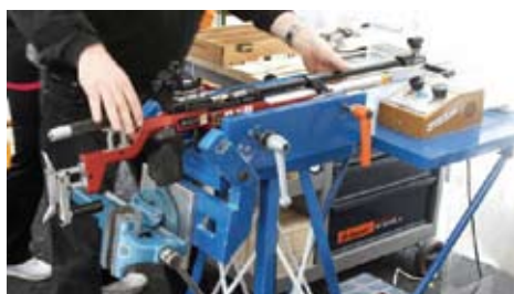
This is the vise used by RWS at their test stand at Hochbruch, the 1972 Olympic range in Munich. It grips the individual parts of the rifle. The legs are screwed into concrete. Note that there is a standard bench vise at the rear that can be swung up and locked into position for air pistol testing.
